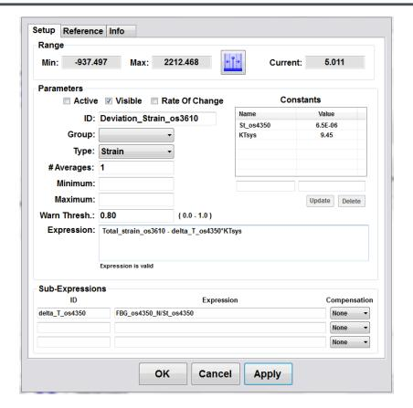
And of course, the os4350 can output absolute temperature, these steps result in the following measurement outputs from the os3600/os4350.
