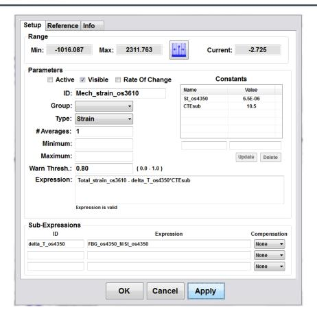
**E. SYSTEM THERMAL RESPONSE** - Strain deviations from typical structural system thermal response can be observed by knowing the substrate temperature and deducing an effective thermal response coefficient of the system.
