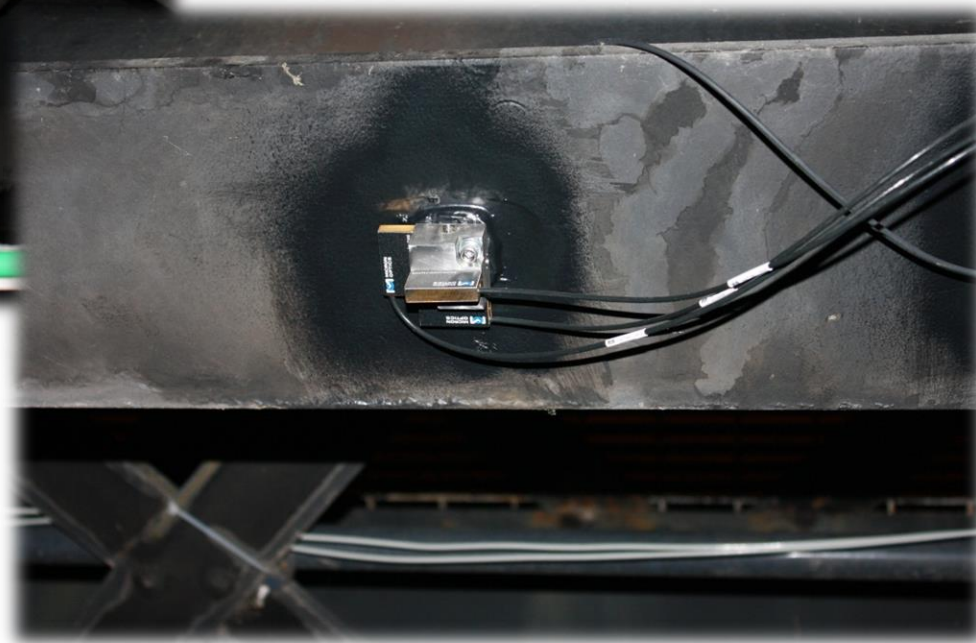
3D Accelerometer being installed on the swing span
